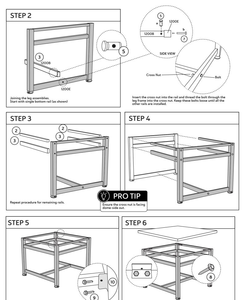
Screw the benchtop to the frame using the timber hex head screws Screw the benchtop to the frame by screwing through the angle brackets into the bottom of the bench. Remember to centre the benchtop to the frame. The benchtop is heavy. You will need another person to assist.
