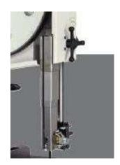
Heavy Duty Rack and pinion lifting system for the top guide unit with telescopic blade protection.
